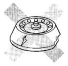
Visually inspect rotor for damage such as dents or chips from being dropped. If the rotor is damaged, do not use the centrifuge and call for service.
