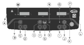
**3.** There are six modes in stirring related to the stirring direction that can be selected by pressing "Six Mode" button **(E)**.
