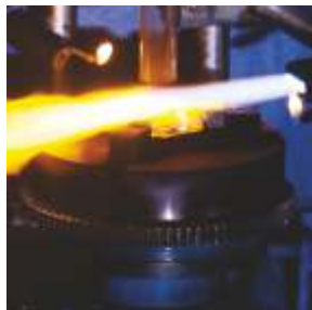
AUTOMATIC CYLINDER FORMING MACHINE : 800 pcs per shift
